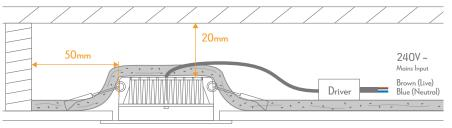
The LED driver is NOT suitable for covering with insulation material.
