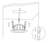
3. Connect the downlight with driver, hold back the spring clip then push the downlight into the hole.
